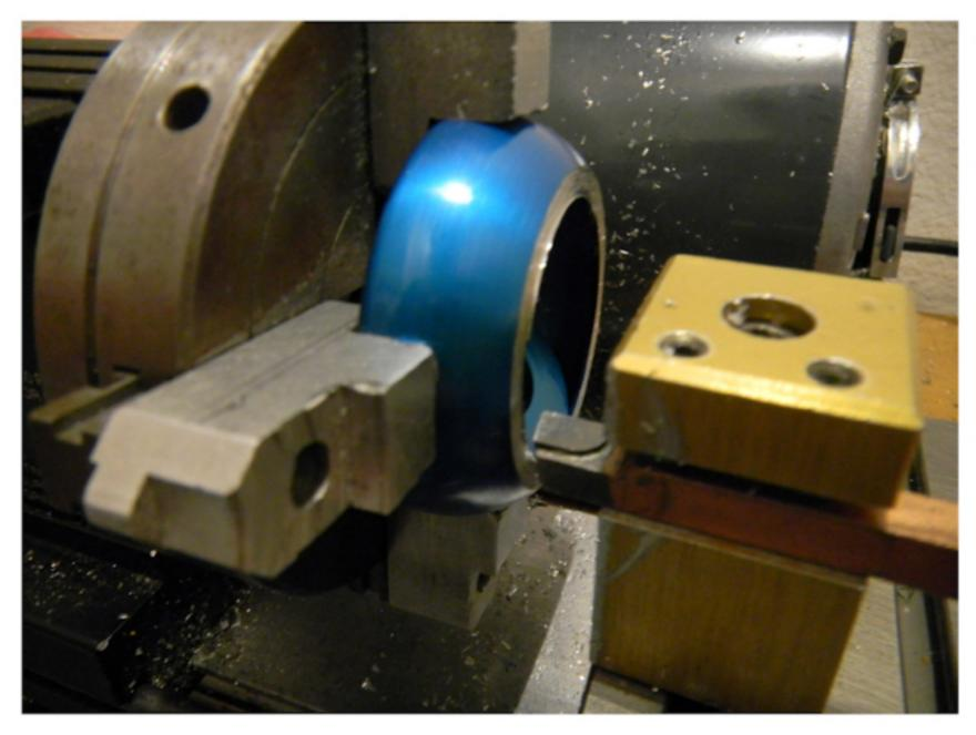
The hub was removed in a slightly different manner than usual. Normally I punch through the yoyo from the front, but I wasn't sure how large of a hub section I would need.
