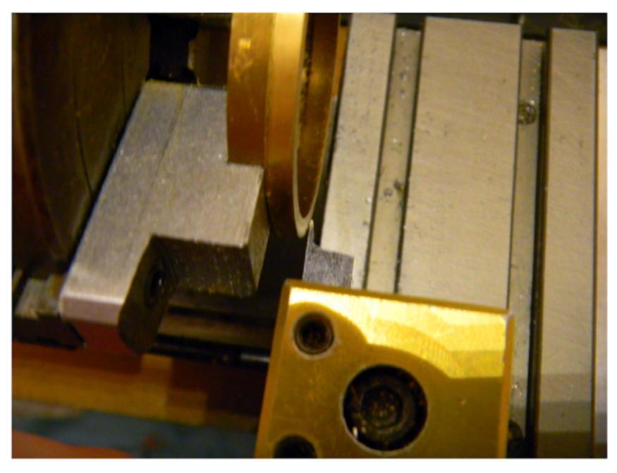
The newly machined brass section is parted off with a very, very thin bit.
