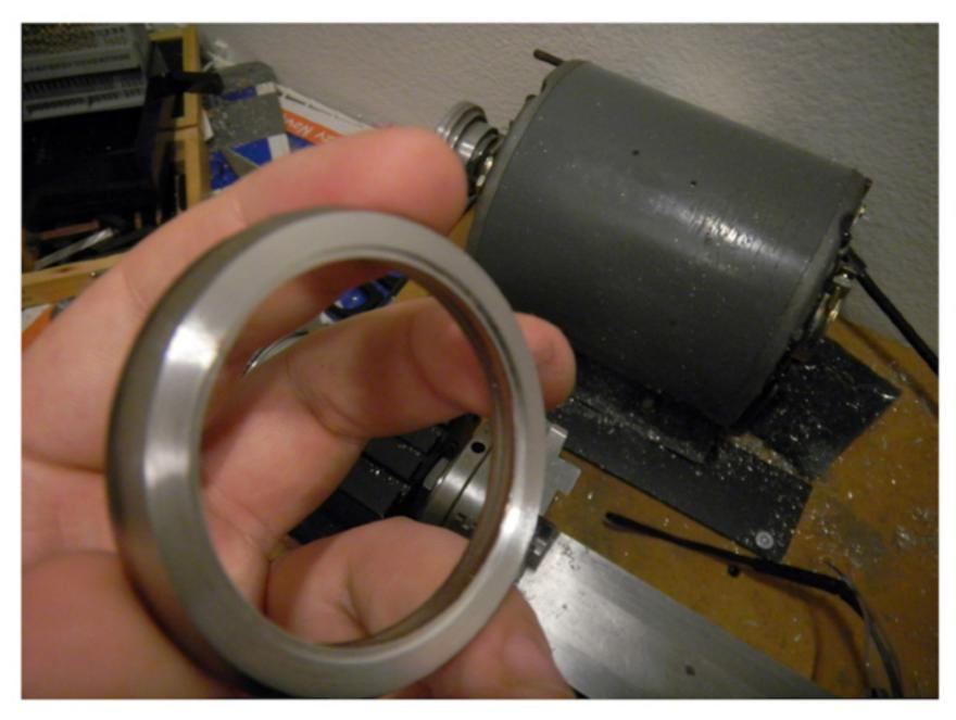
The rim was machined smooth, some width was removed, and a step was cut similar to those cut for the hub.
