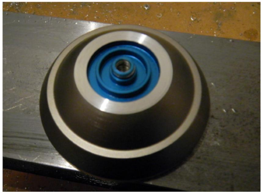
The hub pressed into the Skywalker body.
