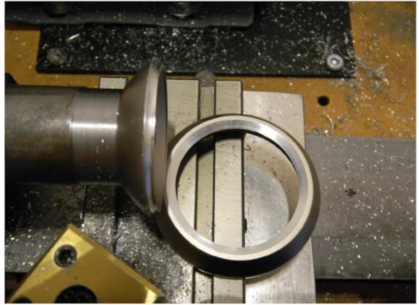
The angle of the cut allowed a larger, thicker section of the rim to be preserved, removing as little material as possible between the shell and rim.
