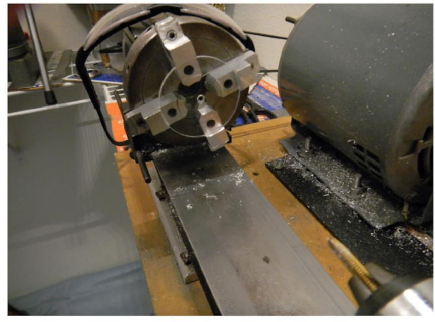
An acrylic disk is mounted, then drilled and tapped with an 8-32 thread.
