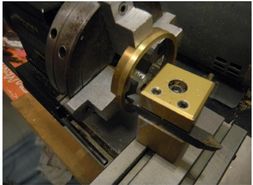
A brass tube is machined to size.
