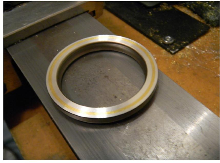
A groove is cut in the rim to match the new brass weight ring.
