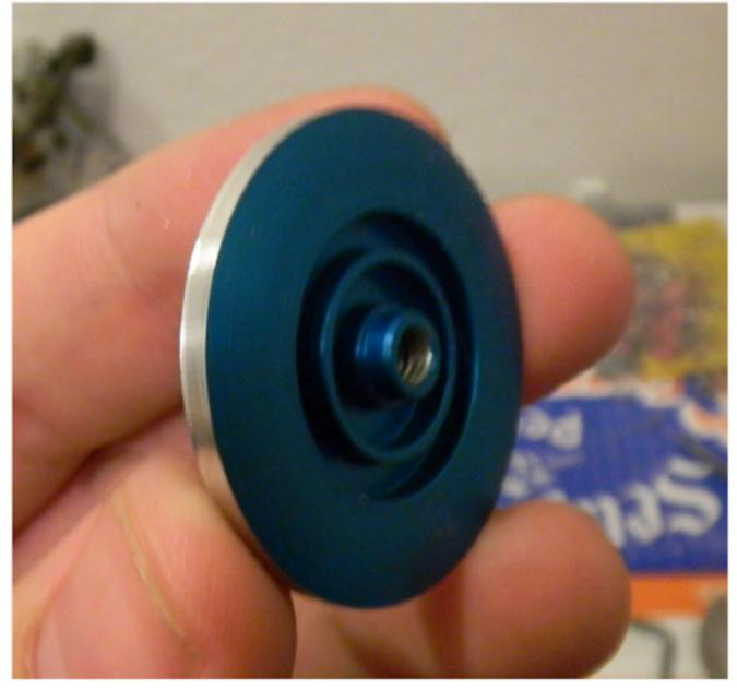
The cut out hub, cleaned up and ready for a step to be cut. This diameter was ultimately reduced to make a smaller hub.
