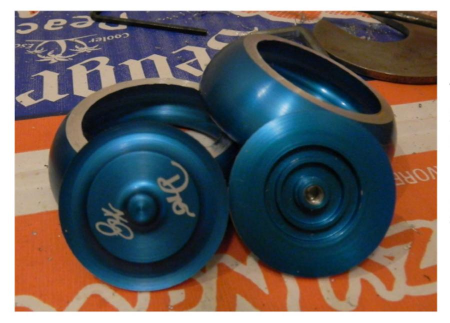
The two removed hubs. You can see the flat surface of the shell where I removed material to release the hub section.
