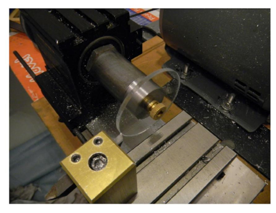
The piece is then screwed onto a piece of threaded rod, which is then tightened down on by a thumbscrew. This pulls against a nut on the other side of the headstock, creating a 'draw-bar'.
