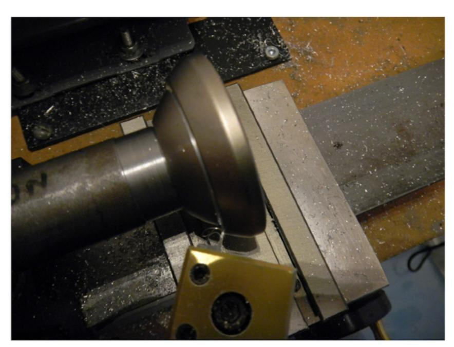
The rim of the Skywalker was removed at an angle to make the cut as short as possible.
